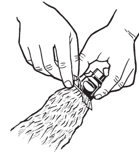
Attach the oven tube to the valve
