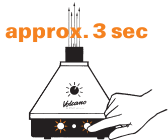
Preheat substance when yellow control lamp is off
