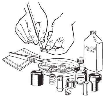
Manual cleaning with alcohol (min 90%)
